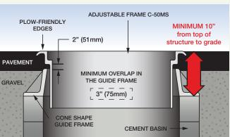
NOTES: The Cone shape guide frame must not be situated in the pavement.
